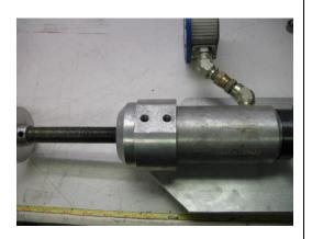
Slide the cylinder over the load pin roller (center roller)
