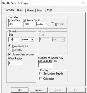
straight line counter check box. Clear the straight line counter check box if the line diameter
