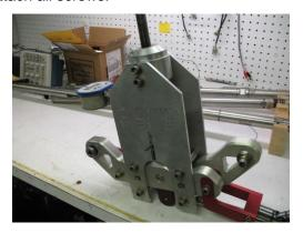
Position the jaw of the cylinder centered over the roller and screw it down until it just contacts the roller. Remember not to put any pressure on the roller while performing the low end.
